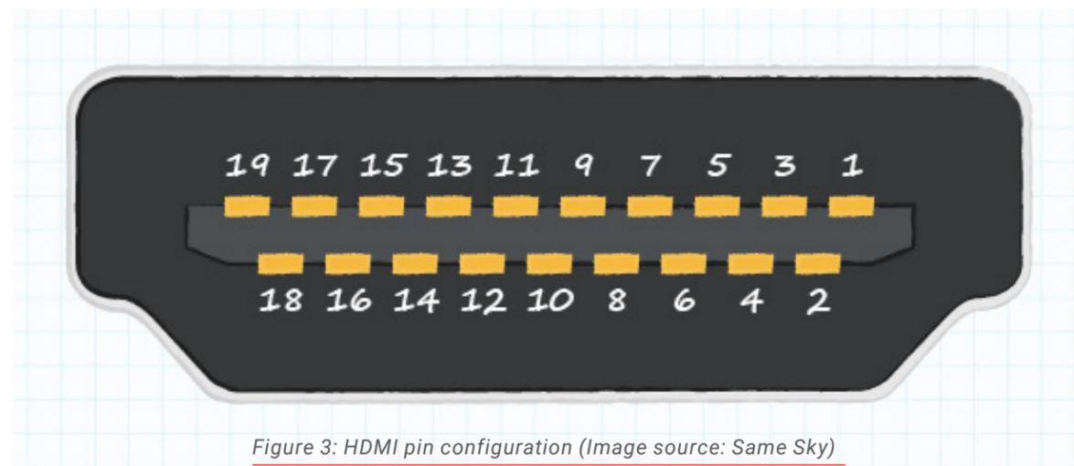
Figure 3: HDMI pin configuration (Image source: Same Sky)
