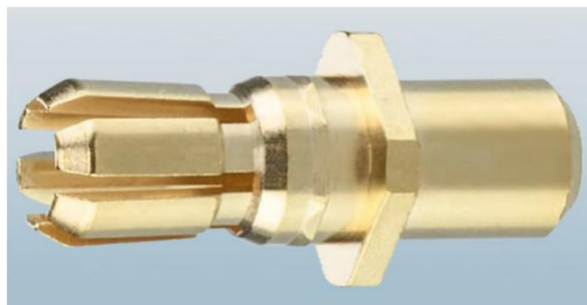
Figure 2: The six-fingered male contact provides positive normal spring force against the interior walls of the female contact to ensure a good connection even in the presence of shock and vibration. (Image source: Harwin Inc., modified)
