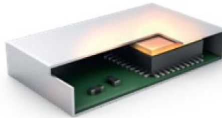
Figure 3: Functionality of a gap filler on an IC.
