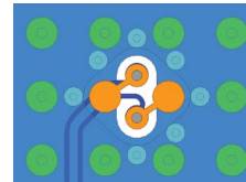
Initial Differential Via Design
